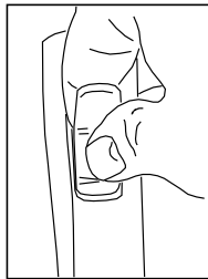
a. Pry dust cover from body.
